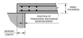
Figure 2 - End bearing configuration
