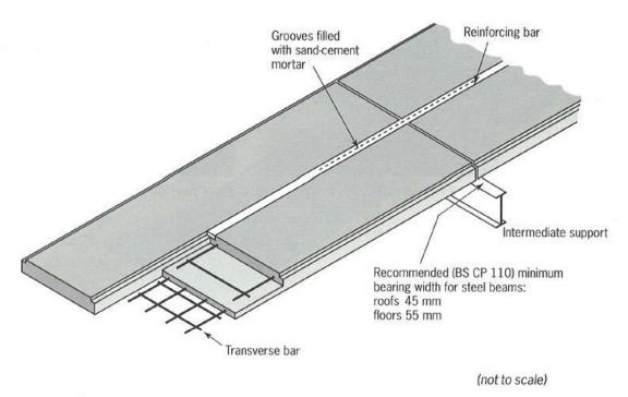
Figure 1 Typical configuration of reinforcement
